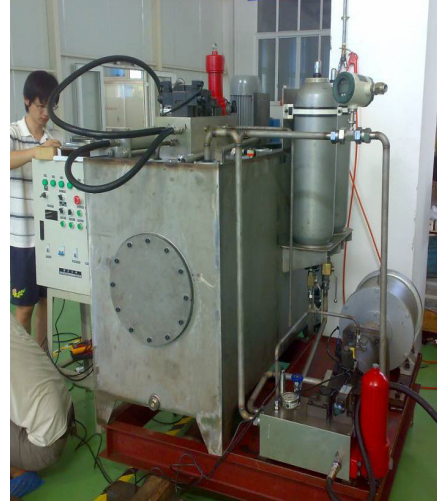
Figure 6: Principle and photo of the hydraulic pitch system
