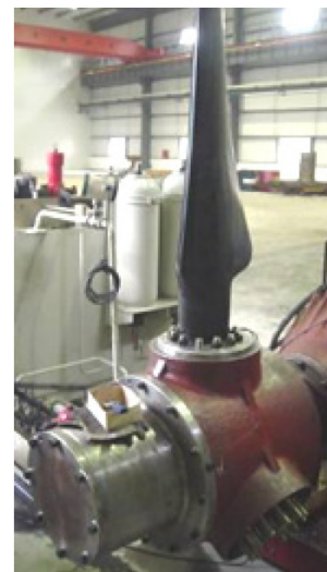
Figure 5: (a) Rotary hydraulic joint, (b) Test of the pitch system
