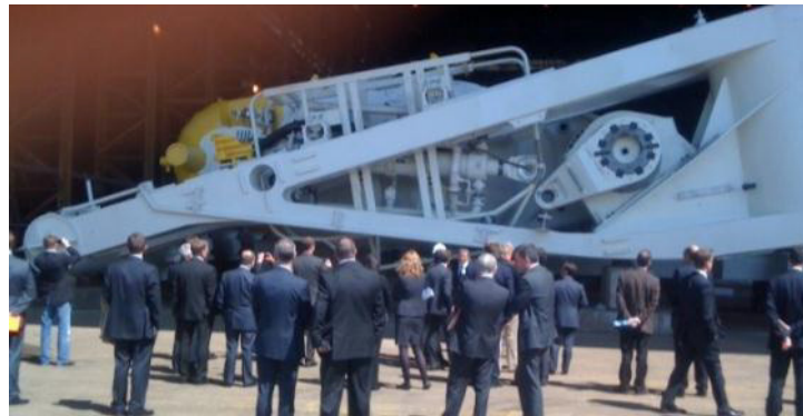
Figure 4: The cylinder module within Oyster 800
