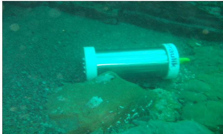
Figure 9: Test piece with Ultraplate layer in the North Sea
