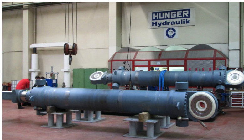
Figure 7: Oyster 800 cylinders on the hydraulic test rig
