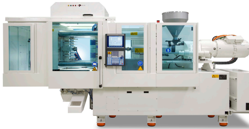
Figure 4: Hybrid injection moulding machine design KraussMaffei CX Hybrid /2/
