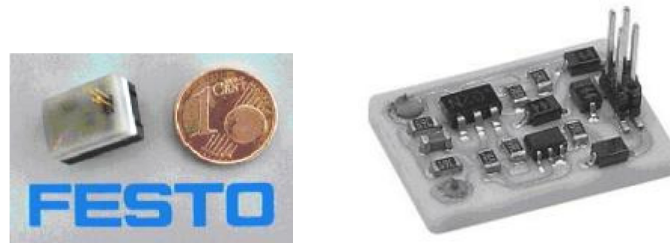
Figure 13: Micro- Piezo- Valve (source: Festo, IMSIP /19/)
