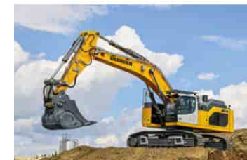
Liebherr R 9XX H2 crawler excavator with hydrogen engine (prototype)
