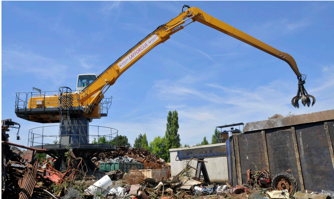
Figure 5: Electric Material Handler (Source: Liebherr)
